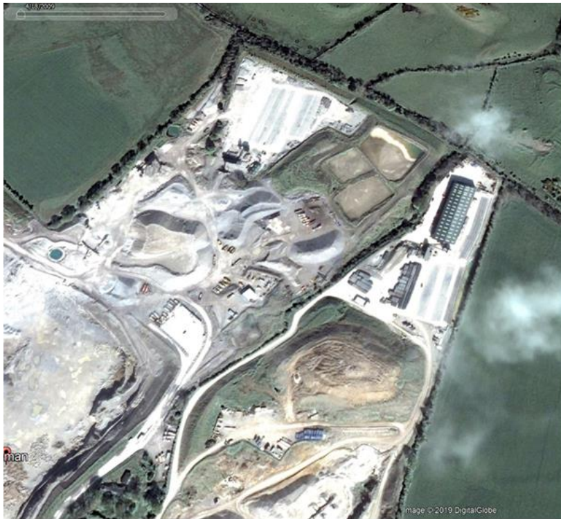
Figure 2.1 – The northern section of Tromman Quarry on 18 April 2009. Note that none of the additional structures listed have been built but the paved ground is visible. Source: REIAR (2019)
